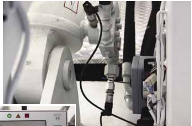
Two Load Systems International LMI pressure transducers were installed on this crane’s hydraulic system. A wireless transmitter (the gray box in the picture above) sends load data from the transducers to the model GS820 display, which shows the LMI load/geometry data.
