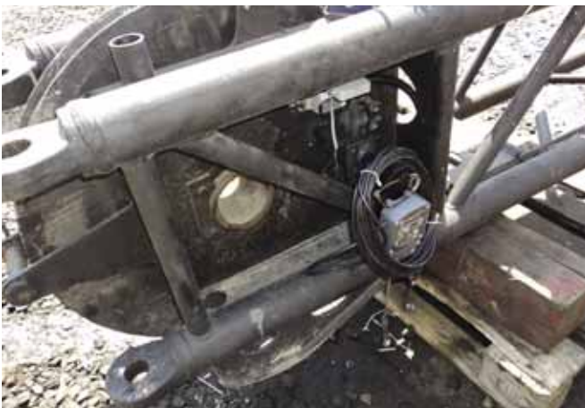
Bode Technical Services installed this new anti-two-block system and switch for a customer.
